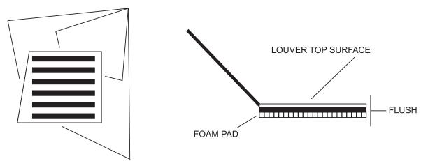
Apply foam pad to entire perimeter of the louver on the back side. Install the pad flush with the edge for best appearance.
