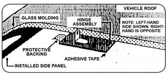
Place the louver on the window with the leading edge of the top slat as close to the window molding as possible and centered side to side. Using a soft lead pencil, mark lightly on the molding the location of the two hinge holes at the top of the louver. Then mark the location of the two tie down studs at the lower outside edges. When all four marks have been made on the molding, take the louver off the window. (On cars without edge molding on the glass, use a crayon and mark the glass-itself).
