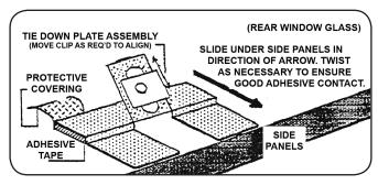
When all attaching hardware has been 'tacked' in place, re-set the louver on the car and fasten the hinges and 1/4 turn tie downs.
