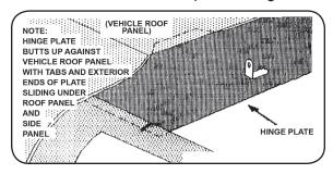
4. Fold back the protective adhesive covering on tie down plate (see below diagram). Position the tie down plates on the glass in the lower corners, sliding the "feet" of the tie downs underneath the side panels. Do not "tack" the tie downs in place until Step 5.
