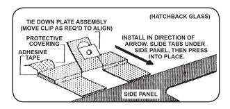
5. Place the louver on the window so that the foam padding rests on the side panels. Turn the fastener in the louver into the mating part located in the tie down assembly. Adjust the position of the tie down as necessary to align and temporarily secure the tie downs to the glass by applying pressure to the exposed portion of the adhesive tape.
